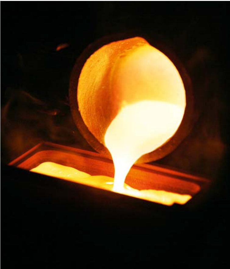
The gold is cleansed of impurities and residues and then processed further in the required purity into bars or other products.
