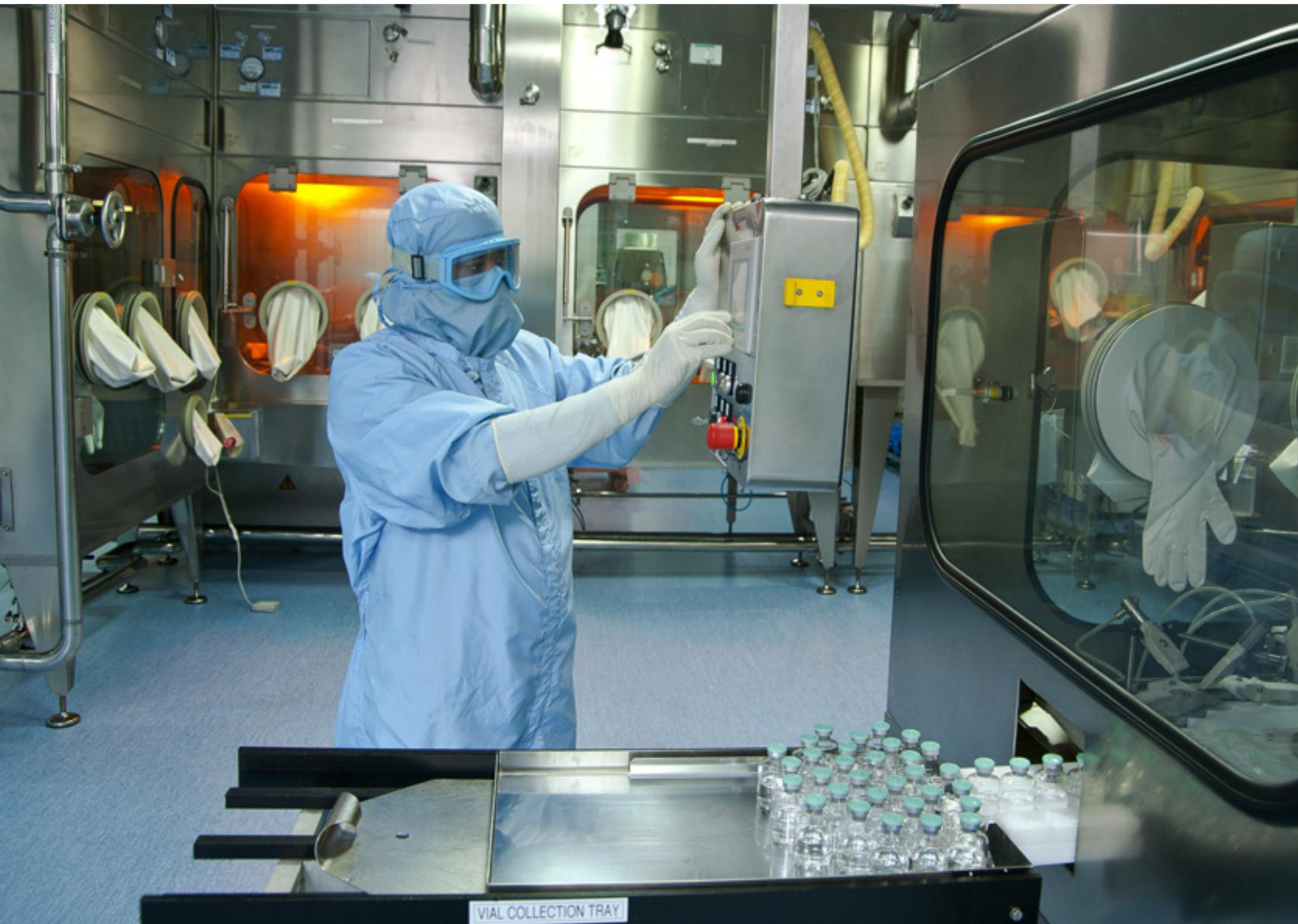
Integrated aseptic filling line with isolator barrier technology in Dr.Reddy's injectable's facility.
